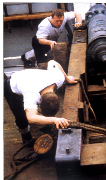
BELOW The same Royal Navy crew have loaded the piece and are now attempting to run it back up to the gunport. Unlike the English four-wheeled truck-carriages, the Spanish relied on these far more cumbersome two-wheeled sea carriages. (Dr Colin Martin)
